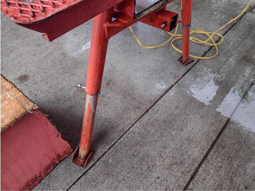
5. Raise the front and set the front jack supports. Insert the pin to hold the jack. Note the wheels are off and the hydraulically operated jack is retracted.
